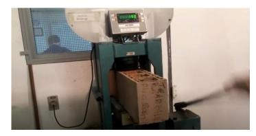
The compression test also obtained good results, proving the strength of the recycled mortar.
