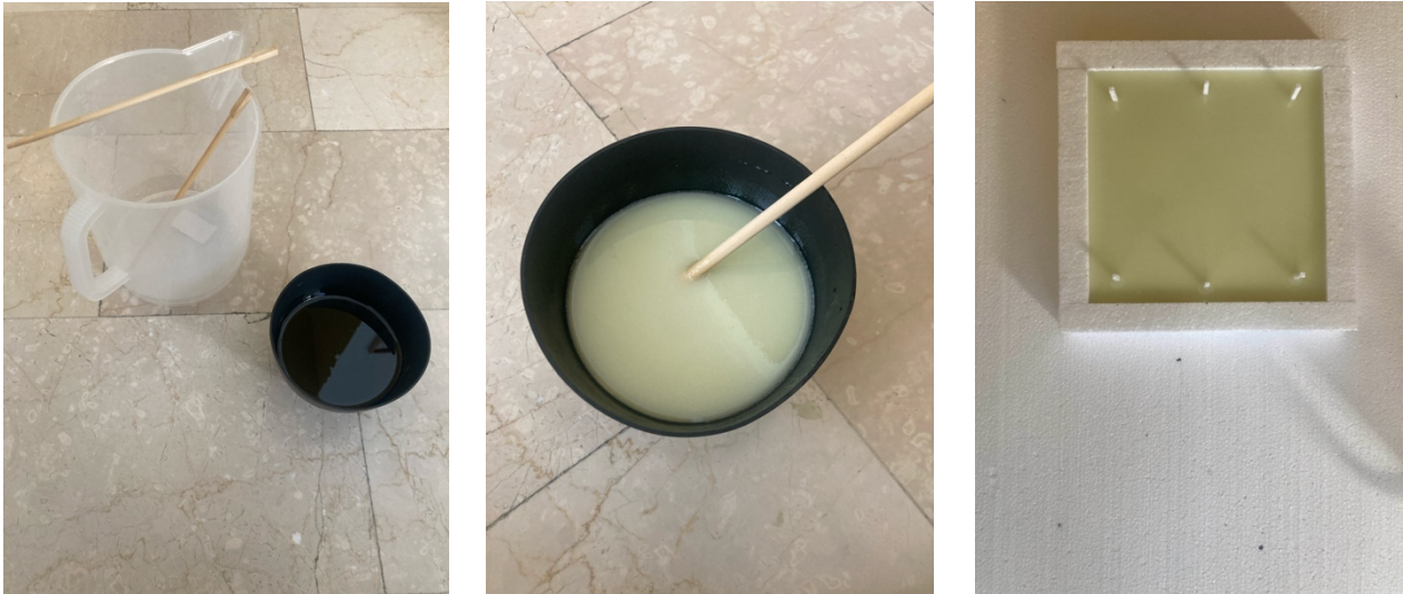
Figure 4. Photographs showing the preparation of the first mould. The manufacturing was deliberately carried out with simple tools and not in a laboratory to demonstrate that the construction process can be done anywhere and by people with no experience. The polystyrene was cut with a blade.
