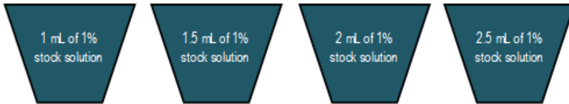
Figure 50: Examples of jar testing buckets with increasing volumes of stock solution
