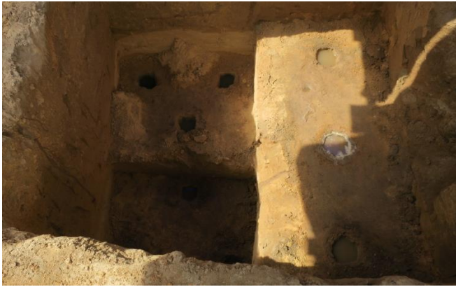
Figure 56: Percolation test step digging, Source: MSF Nigeria
