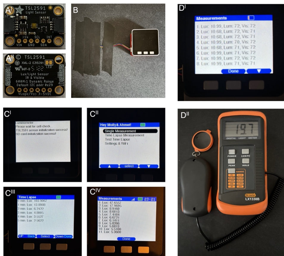
Fig. 8 | A Detailed Setup and Methodology for Measuring the Light Output of Phosphorescent Panels Using a High Dynamic Range Lux Sensor and ESP32 Microcontroller
