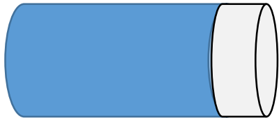
200 mm diameter White PVC hollow pipe with pipe cap and one side open
