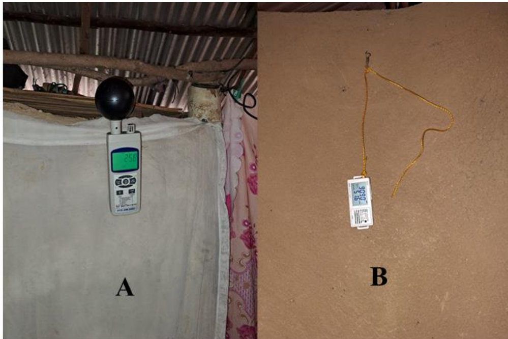
Figure 7: Picture of temperature and humidity data logger, A showing Wet Bulb Global Temperature (WBGT) data logger and B showing HOBO data logger.
