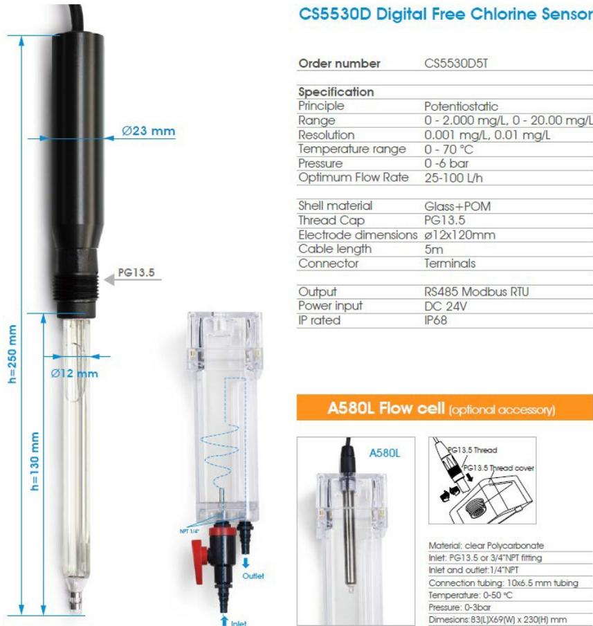
Figure 1: Main specifications and dimensions of the selected sensor (\*offered only with range 0-20mg/L and opt. flow rate 10-30L/h).
