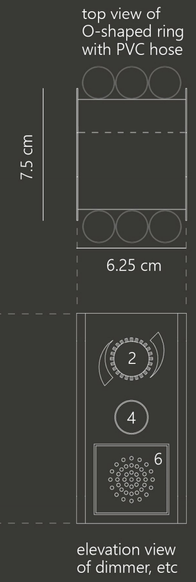
light dimmer + motion sensor + panic button + circuit board for emergency alarm in O-shaped ring
